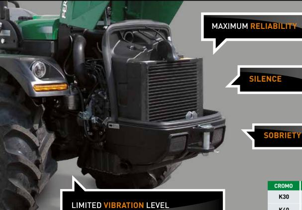
The Cromo are moved by two latest generation engines: a 26 HP three cylinder engine and a 35.6 HP four cylinder engine, both with indirect injection and natural aspiration.
